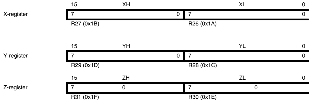
Figure 5-3. The X-, Y-, and Z-registers
